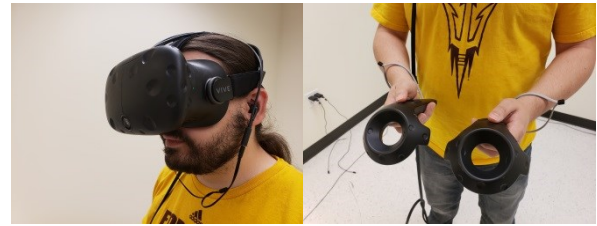
Figure 2. Close-up of HTC Vive equipment. Left: Headset and earbuds. Right: Vive controllers with vibrotactile feedback capabilities to simulate feeling the rumble of the crowd.
